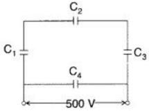
Q71) A network of four capacitors each of 15μF capacitance is connected to a 500 V supply as shown in the figure. Determine: (a) equivalent capacitance of the network and (b) charge on each capacitor.
